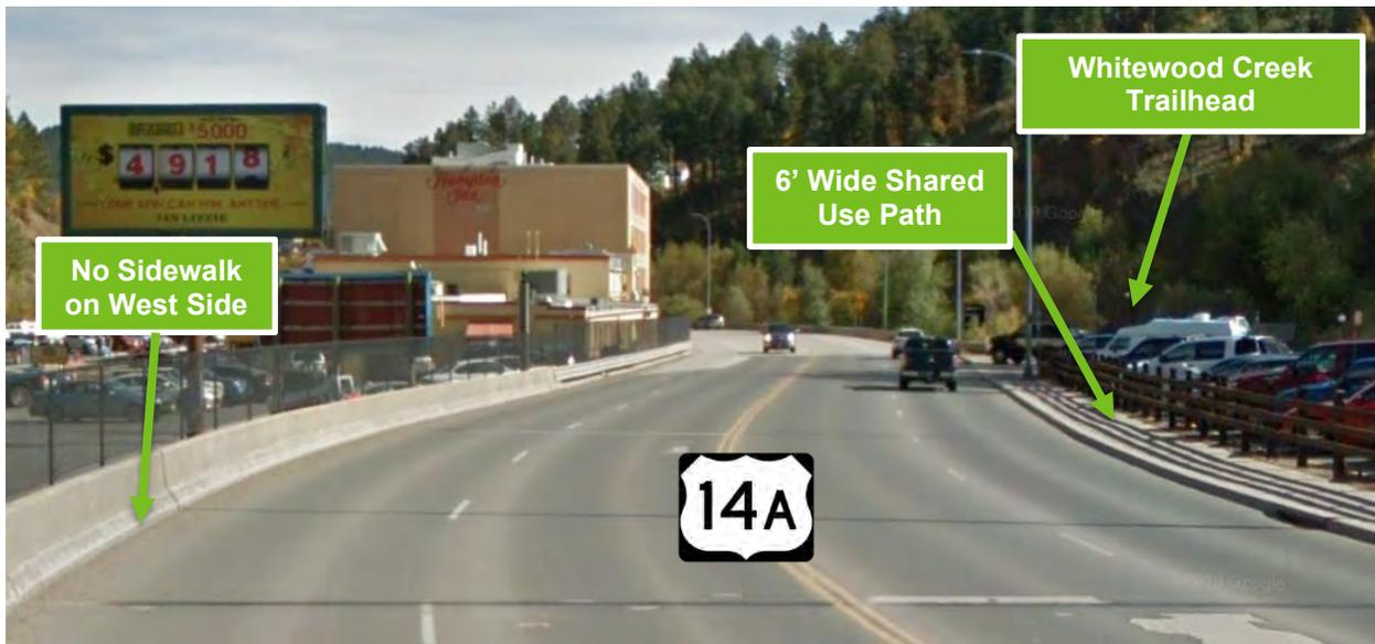
Figure 22. Shared Use Path Designation on US14A East Sidewalk (Facing North)
